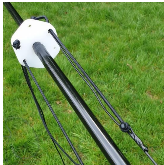
80m tension (right) to very top spreader
