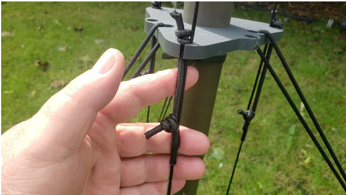
Picture of the 1 st Spreader with all elements fitted
